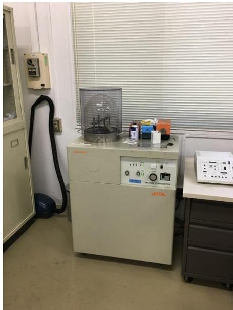
Figure 8. Carbon coating equipment.
