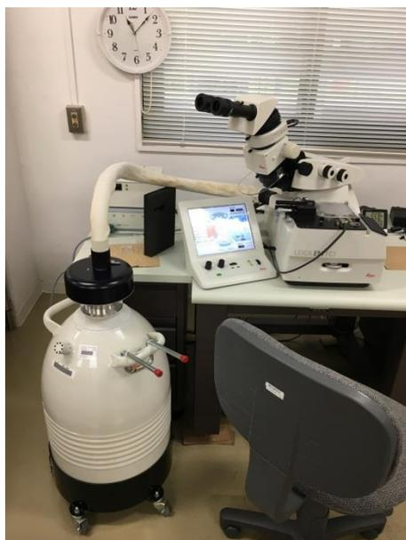
Figure 6. Ultra-thin cryo-sectioning equipment.
